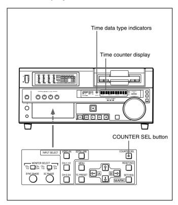
Open the door on the lower part of the front panel, and press the COUNTER SEL button.
